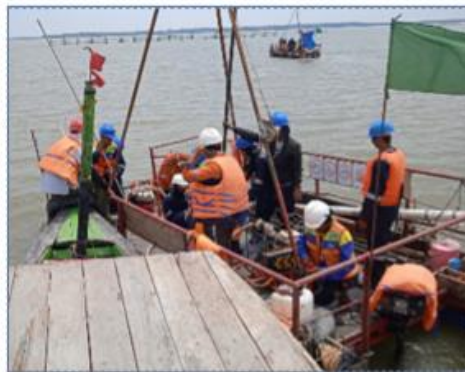
Figure 11. Seismic drilling with catamaran equipment in transition zone
